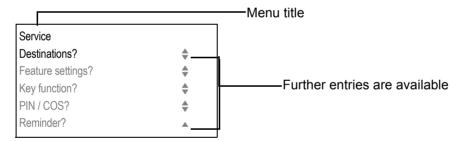
The menu structure consists of several levels. The first line in this structure shows the menu currently selected while the remaining lines show the options for this menu. The arrow next to an entry indicates the availability of additional options for this entry.
