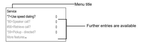
The menu structure consists of two levels. The first line in this structure shows the menu currently selected while the remaining lines show the options for this menu. The arrow next to an entry indicates the availability of additional options for this entry.
