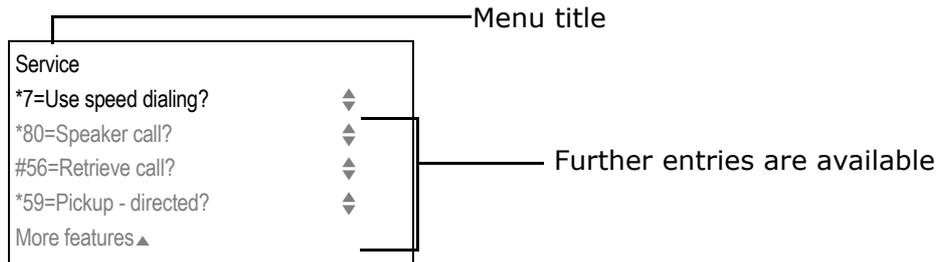
The menu structure consists of two levels. The first line in this structure shows the menu currently selected while the remaining lines show the options for this menu. The arrow next to an entry indicates the availability of additional options for this entry.
