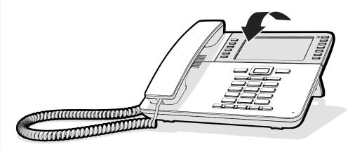
You can tilt the display. Adjust the display unit for best readability. The display snaps into position.
